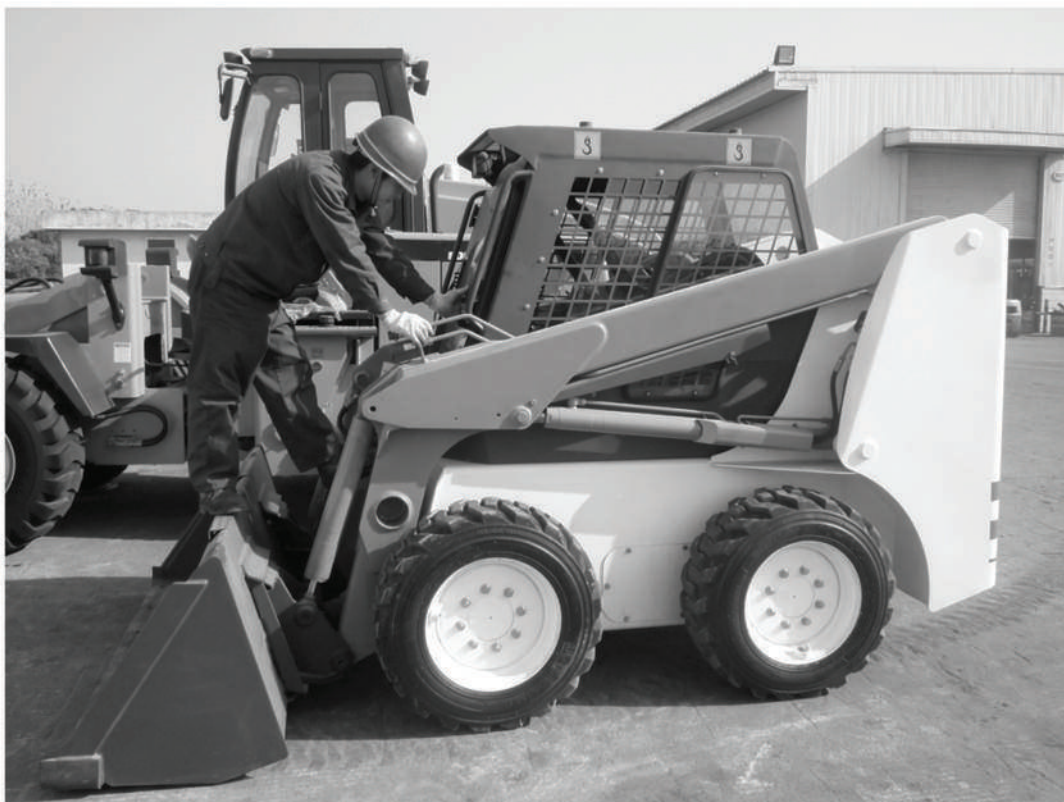
Figure 12 CORRECT WAY FOR MOUNTING THE MACHINE
